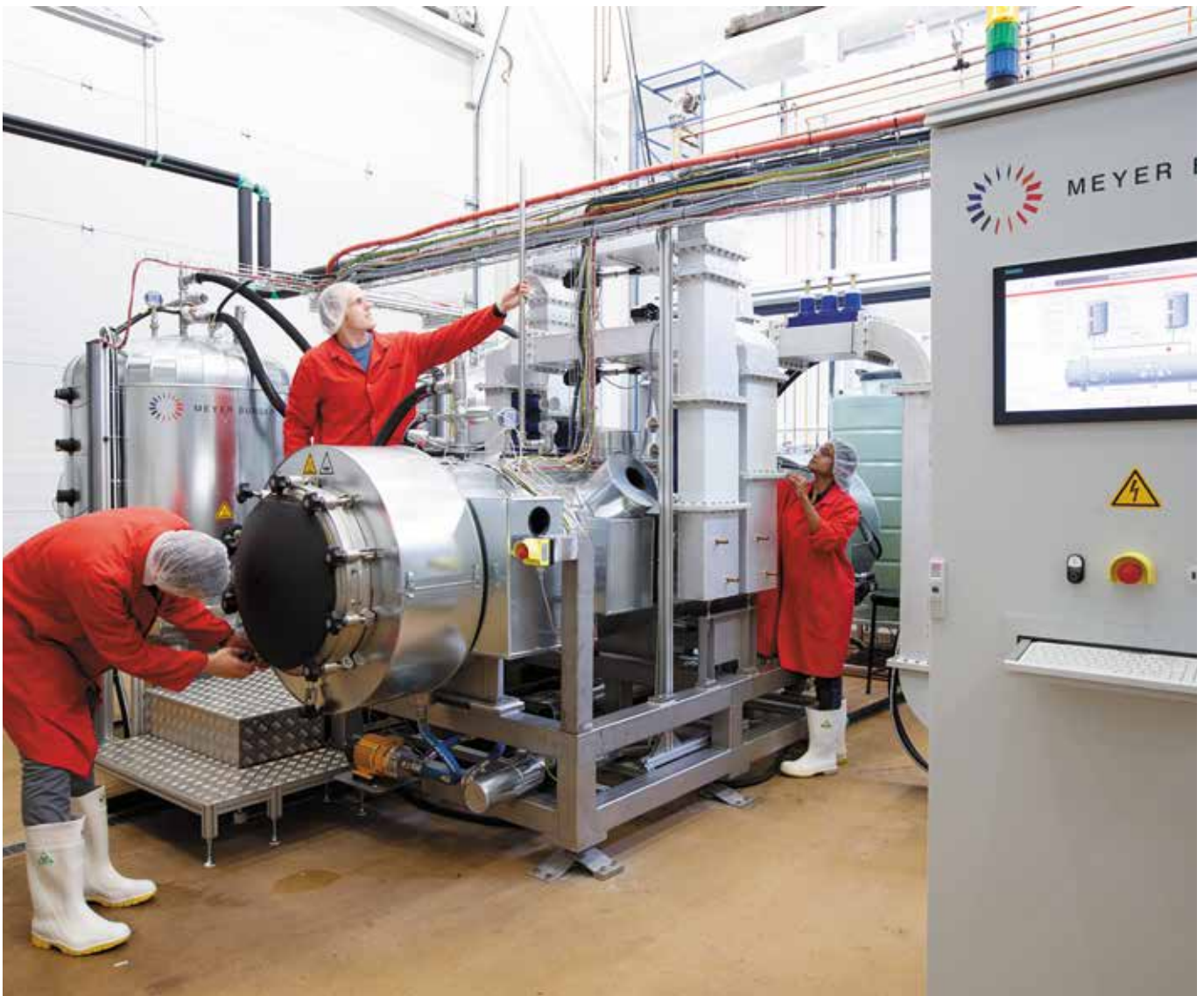
Meyer Burger CiMPAs microwave-assisted processing unit being used in the project
