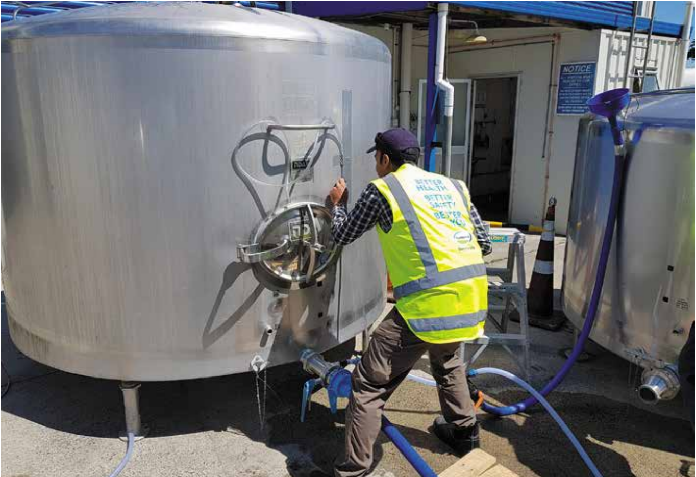
Bal Timilsina testing pump-around agitation in milk vats of different shapes
