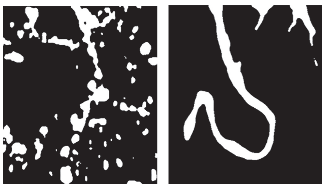
Fig4 - Left: Spray pattern for water with no fibres at the nozzle for P_a=1 bar: ligaments break and disperse into droplets. Right, Spray pattern for 5 wt% wheat fibres in an apple juice concentrate at the nozzle with P_a=1 bar: ligaments remain intact
