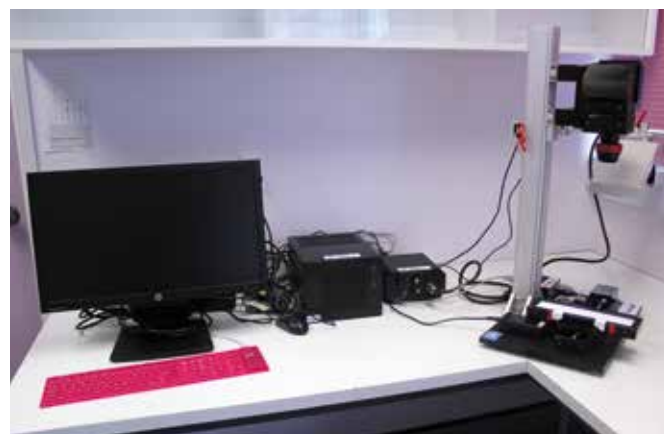
Hyperspectral camera, illumination, sample and computer
