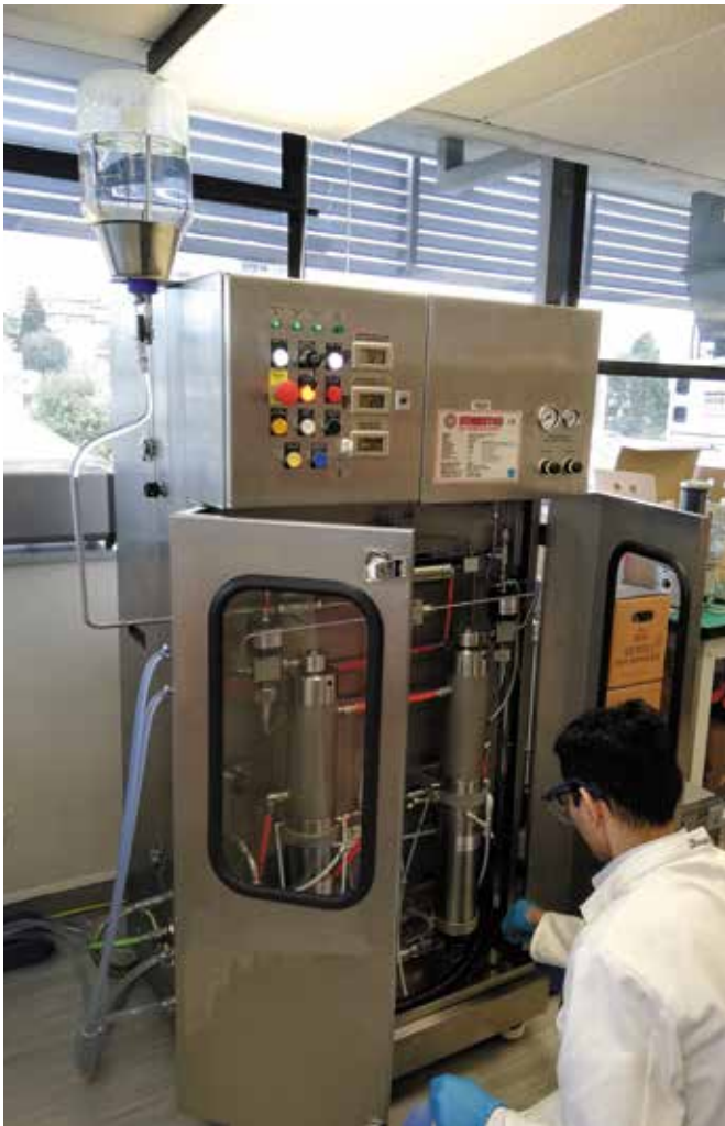
Figure 2: A pilot scale UHPH (420 MPa max) unit at the University of Auckland
